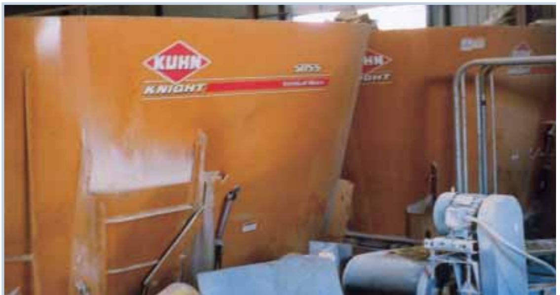
These two mixers at the Grisham Farms were purchased with assistance from the Market Development Program. The mixers, which are about eight-feet tall, hold 11,000 pounds and can process 50,000 pounds of raw materials every hour.
