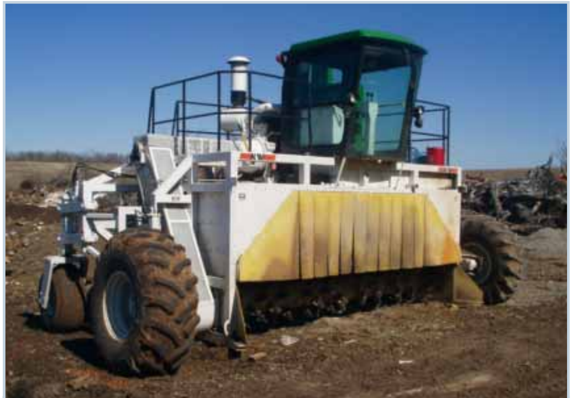
At Black Oak Organics in Verona, this $95,000 windrow turner grinds, chops and shapes windrows that are 14 feet wide and about eight feet tall. The windrow turner, which weighs 36,000 pounds and is about 12 feet tall, can cover a quarter of mile in an hour.
