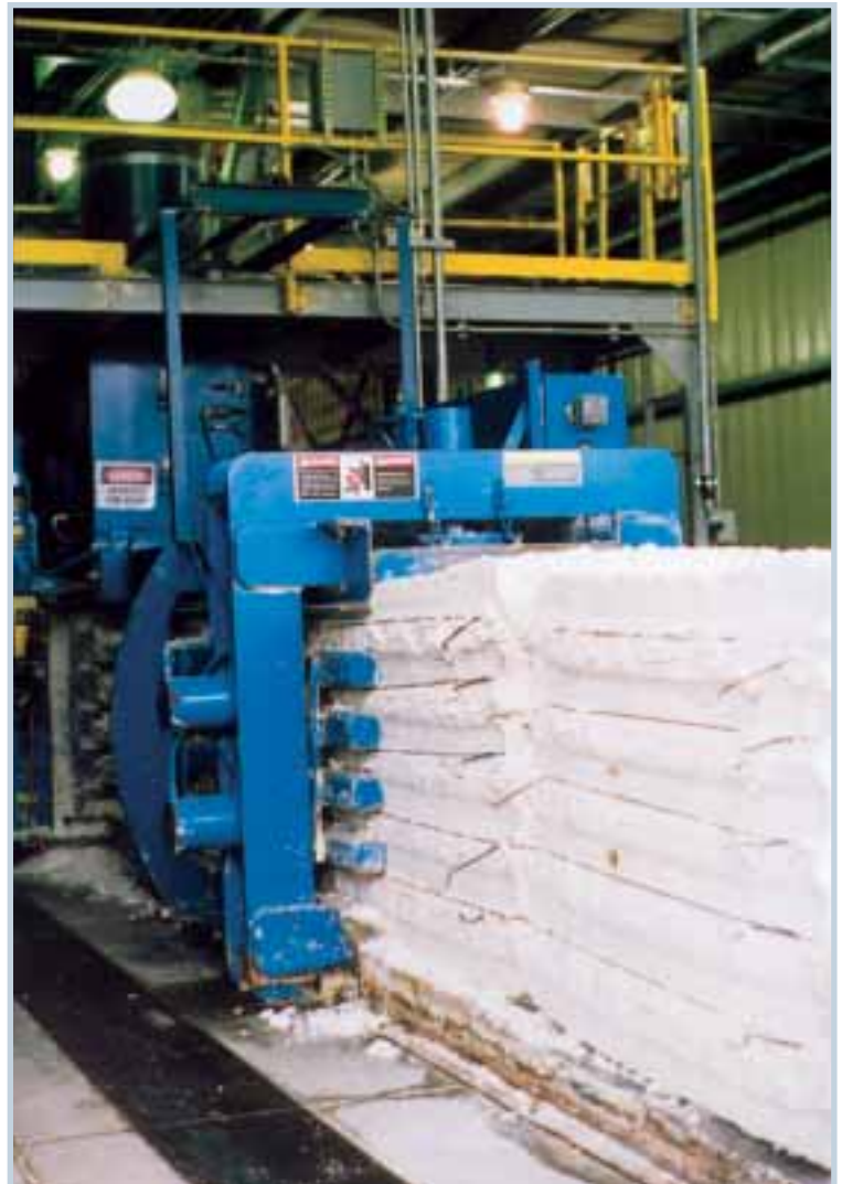
Company officials at Procter & Gamble purchased this blue baler with financial assistance from the Market Development Program. Every hour, the baler produces one three-foot bale of diaper dust that weighs 600 pounds. Later it is shipped to another company for reuse in a manufacturing process.
