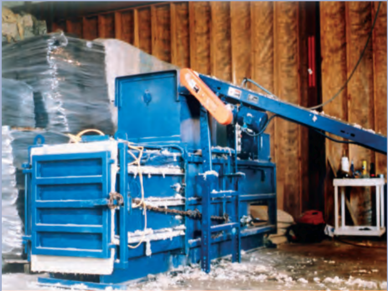
This blue machine receives waste carpet from a conveyor belt and then produces a 300-pound bale. The scrap carpet is shipped to end users and reprocessed and used for numerous plastic products, including boat docks, highway culverts, and the black covers for car radiators and motor fans.
