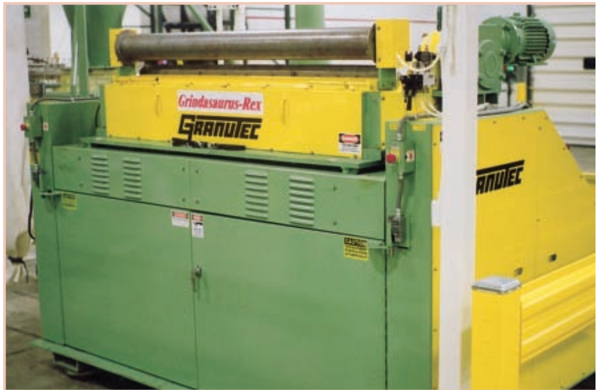
Nike IHM received $50,000 from the Missouri Market Development Program to purchase this granulator. Nicknamed “Grindasaurus-Rex,” it weighs 2,300 pounds and is seven feet tall. The granulator can grind 2,000 pounds of plastic per hour and operates 24 hours a day, seven days a week.
