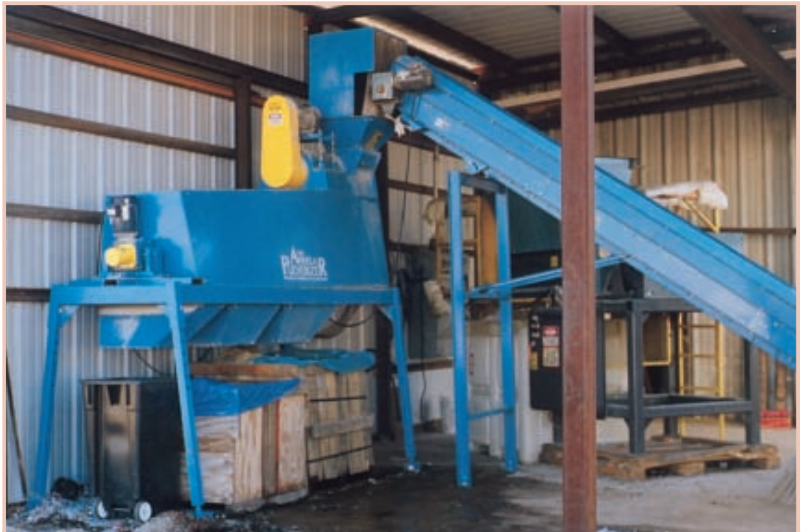
Laclede Industries, Inc., a sheltered workshop in Lebanon, received $49,287 from the Market Development Program to purchase a glass crusher. The big blue glass crusher weighs 4,600 pounds and can grind 20 tons of glass per hour. The crusher was purchased from a St. Louis-area company and cost $11,000 to ship it to Lebanon from St. Louis.
